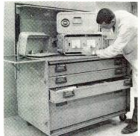
Service bench carries power supply and drawers of tools and spares.
