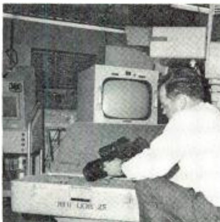
Lens and fittings are cradled in polyethylene-lined compartments.
